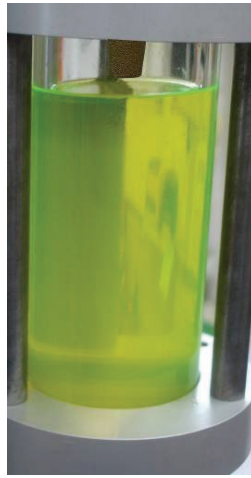
Oil, refrigerant and UV well mixed with each other.
